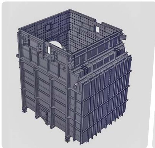
Fig. 5 – 3D model of the diverter box
