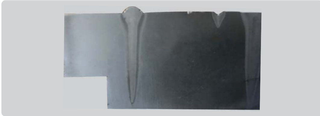
Fig. 6 – Cross-section of the seam welded joint on 07X12HM5Φ-Ш grade pipe sample
