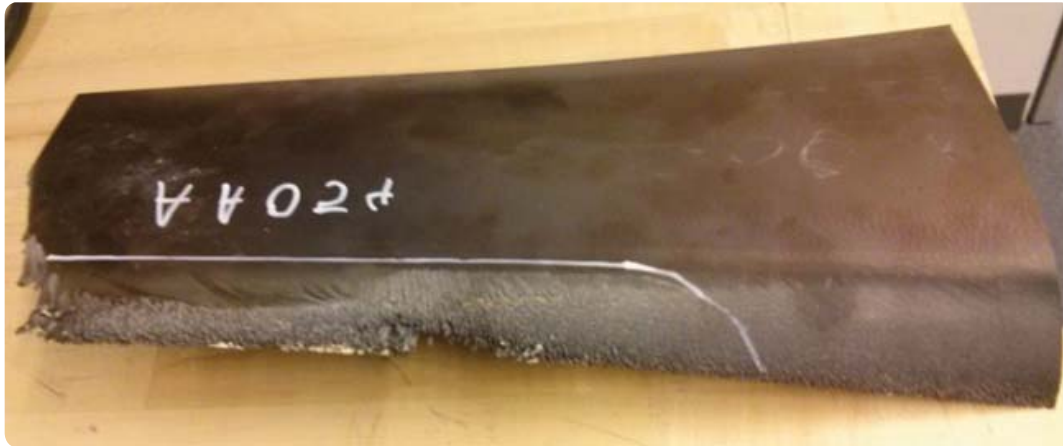
Fig. 2 – Droplet erosion on the leading edge of the last stage blade of a steam turbine (Courtesy of NCCConsulting)
