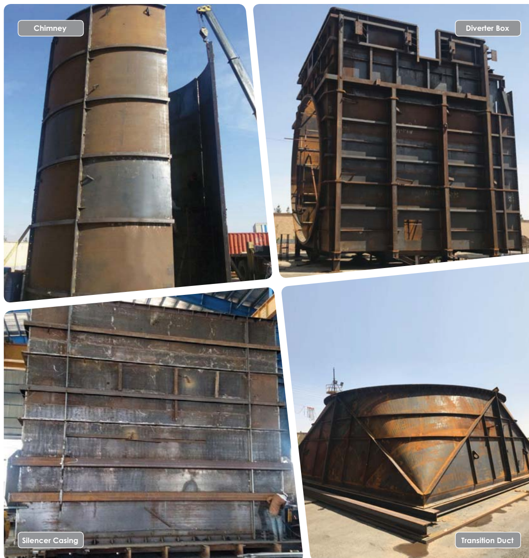
Fig. 11 – MGT-80 gas turbine exhaust system manufacturing process in action
