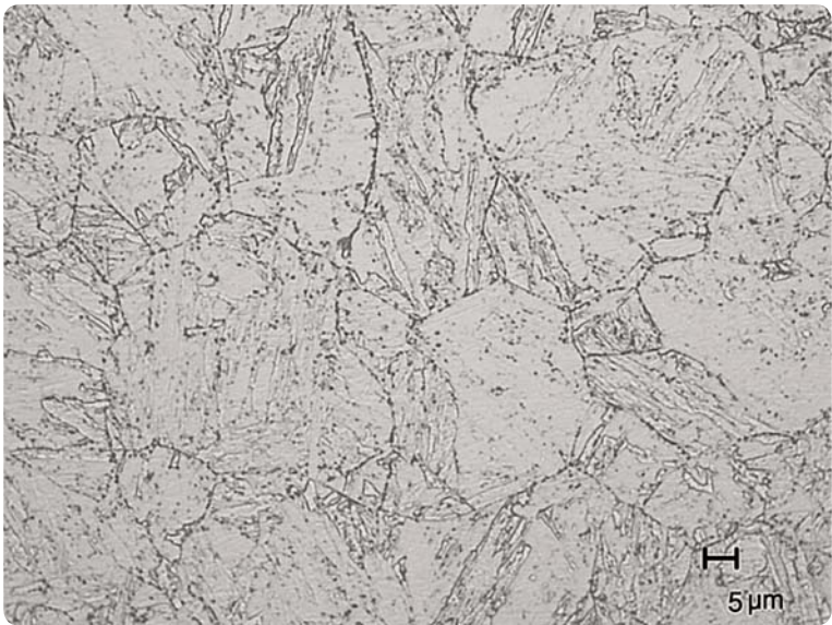
Fig. 1 – Microstructure of the 07X12HM5Φ-Ш (ЭП609-Ш) grade stainless steel
