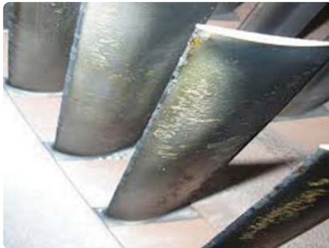
Fig. 1 – Worn compressor blade operating in wet compression system (Courtesy of NCCConsulting)
