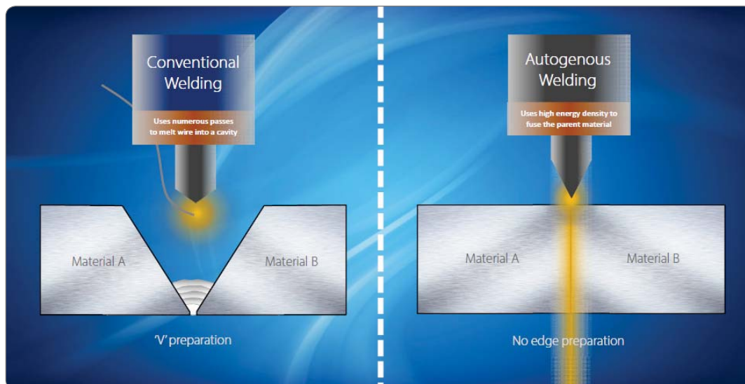
Fig. 1 - Conventional vs. K-TIG welding practices (courtesy of K-TIG, Australia)
